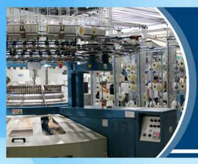
It has a complimentary knitting unit equipped with wide range of fabrics machines. This includes various knitting types like Jersey, Rib, Interlock and auto striper.
